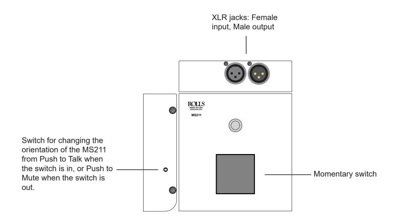
The MS211 rear panel has two screw holes for convenient mounting.
